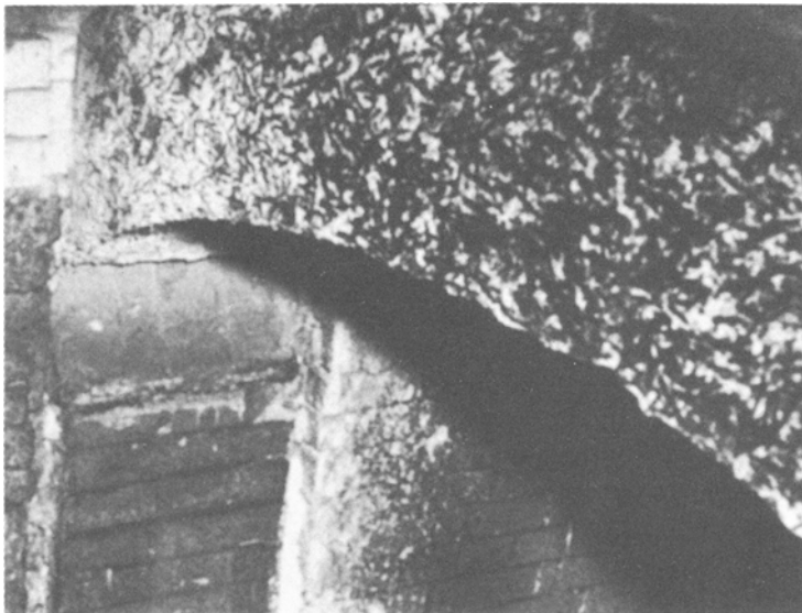
Figure 26 Pre-cast refractory furnace arch reinforced with melt-extracted type 302 stainless steel staples showing three times the life of unreinforced refractory [236].
