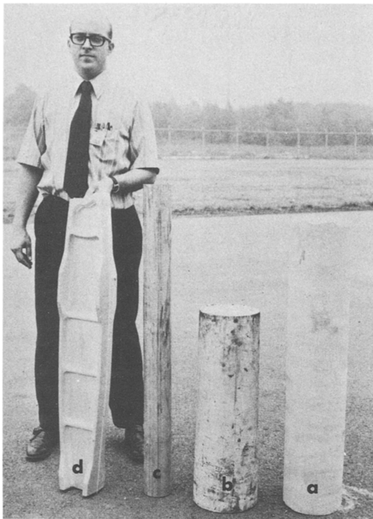
Figure 21 A production sequence for an aircraft forging made from atomized pre-alloyed powder. (a) Cold compact; (b) hot-pressed compact; (c) extruded rod; (d) forging [155].
